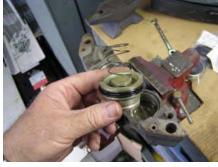
Lube the O-ring with brake fluid and work it back in the bore. Start by angling the piston in the bore and working it with an awl or similar tool. Be careful not to pinch the ring. Work it in. Do not force it.
