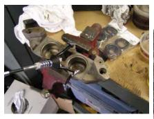
Use a lubricant (brake fluid is ok) and do not hone any more than you need. Keep the hone moving to keep things even. After honing is complete, clean the bores one more time and blow out with compressed air.
