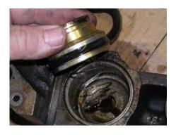
Inside will be a spring, save it, they are not normally in a rebuild kit Repeat the disassembly for the remaining pistons. If you haven't cleaned the calipers do so now. Mineral sprits will work fine.
